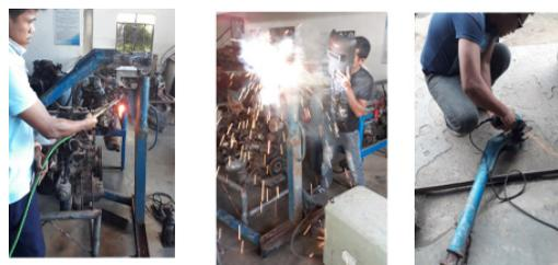
Figure 3. Fabrication of the lifting device using gas arc welding and electrically operated angle grinder.
