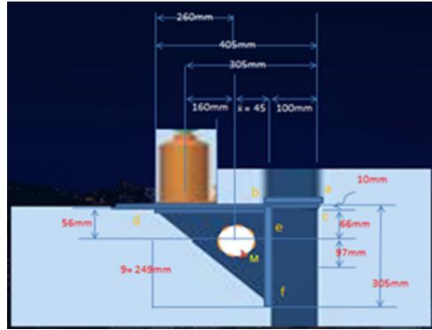
**Figure 1b.** Identified load bearing point in the lifting device where appropriate weld is applied
