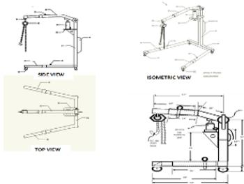
Figure 2. The working drawing of the combined hydraulic and mechanical automotive workshop crane
