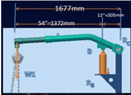
**Figure 1a.** The figure shows the retractable boom is free to rotate around an axis and when a torque or load is applied changes its angular momentum.
